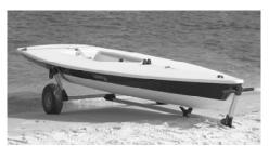
SEITECH dollies are the easy-to-use, light-weight, small boat transportation solution. The Laser dolly has been designed specifically to fit and support the shape of the hull. Special features of the Laser dolly include a rounded bow support for secure transportation and gunwale supports for proper storage. SEITECH dollies allow you to spend less time getting your boat to and from the water and more time on the water.
