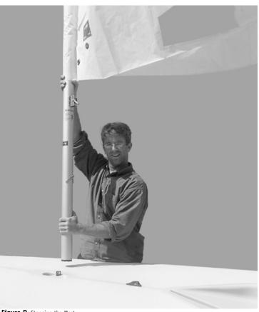
Figure D: Stepping the Mast
