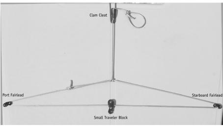
Figure C: Rigged Laser Pro Traveler Line
