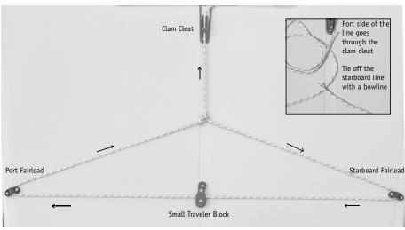
Figure B: Rigged Laser Standard Traveler
