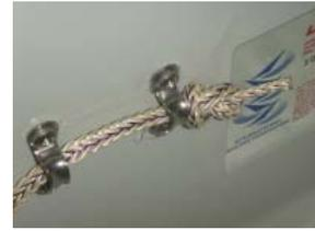
4 Take the 1.2 m length of Vectran V12 and tie a figure 8 knot in one end.
